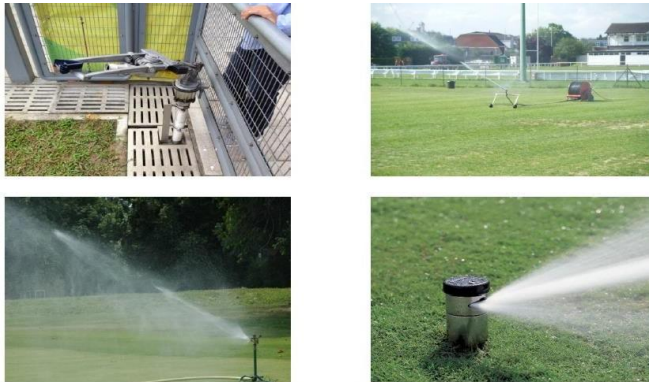
Fig. 3. Types of irrigation systems used in the sports turf industry. From left to right: canon type, self-travelling type, static type and pop-up type. Only automatic pop-up irrigation systems are considered appropriate for pitches
